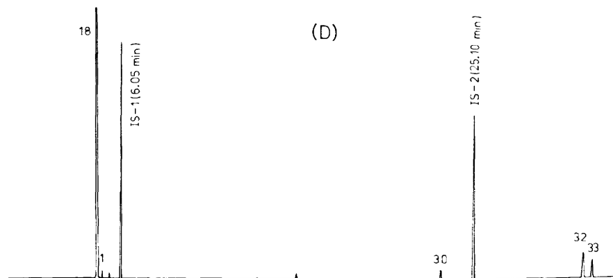
Fig. 3. Gas chromatograms of organic solvent components in typical synthetic resin paints. Peak numbers: see Table I. \text{BrC}_n = branched hydrocarbons with n carbon atoms. (A) Epoxy resin paint; (B) hydrophilic resin paint; (C) phthalate resin paint; (D) water-soluble resin paint.
